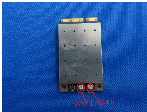
Antenna RF Port Plot
