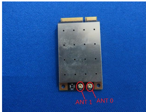
Antenna RF Port Plot
